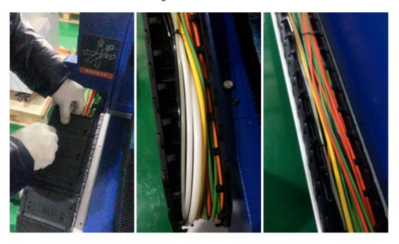
9. Remove the access panel at the end of the Y axis drag chain.
