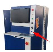
9. (For low power lasers only) Turn on the fiber laser.
